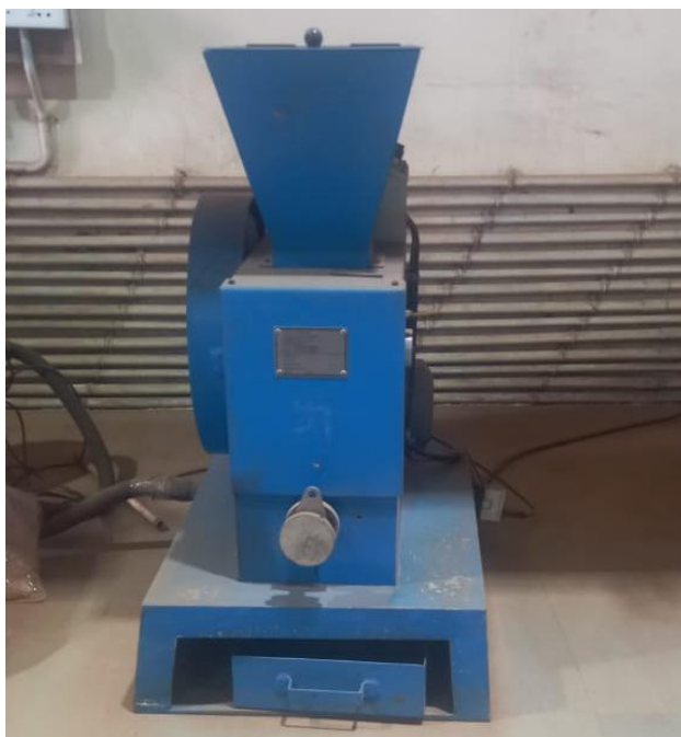
Photo-12.1 Photograph showing sample sample crusher used in sample processing
