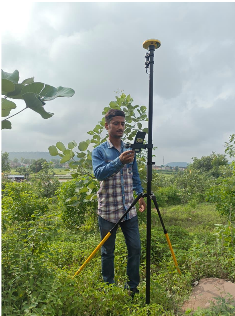
Photo-11.1: DGPS survey in the block using DGPS DA 2 Catalyst System)
