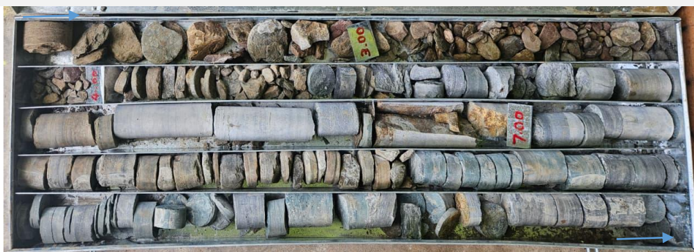
Photo.7.2: Core photograph showing Upper Shale and sandstone member and Glauconitic sandstone member in Borehole MDLH-07
