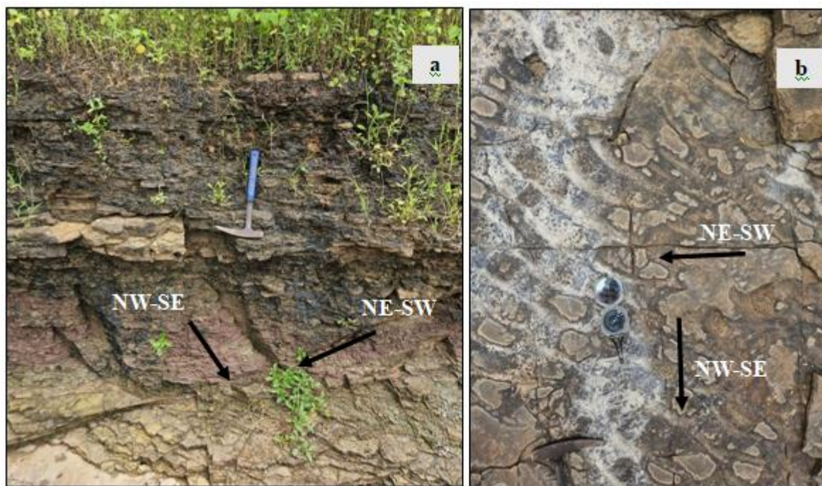
Photo.7.10: Photograph showing of two sets of joints; a) Cross section view. b) Top view
