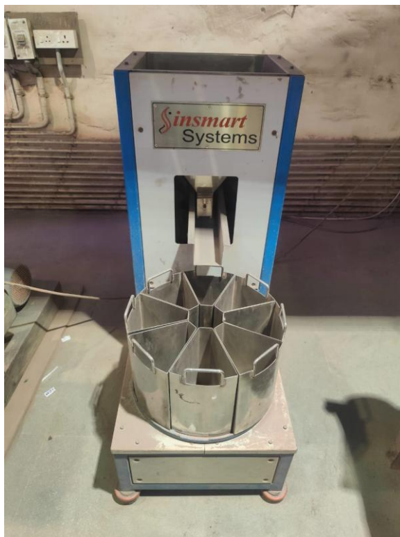
Photo-12.3: Photograph showing coning-quartering equipment used in sample processing
