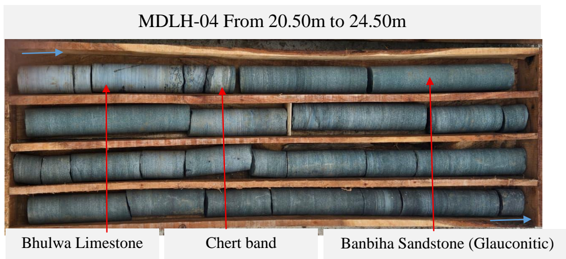
Photo.7.7: Core photograph showing Bhulwa Limestone and Banbiha Sandstone contact, Borehole-MDLH-04 (Depth -20.50m to 24.50m)
