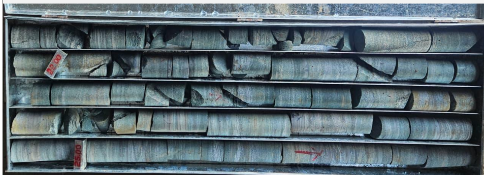
Photo7.8: Core photograph showing Glauconitic sandstone of Banbiha sandstone member in borehole -MDLH-08 (21.00m to 25.80m)
