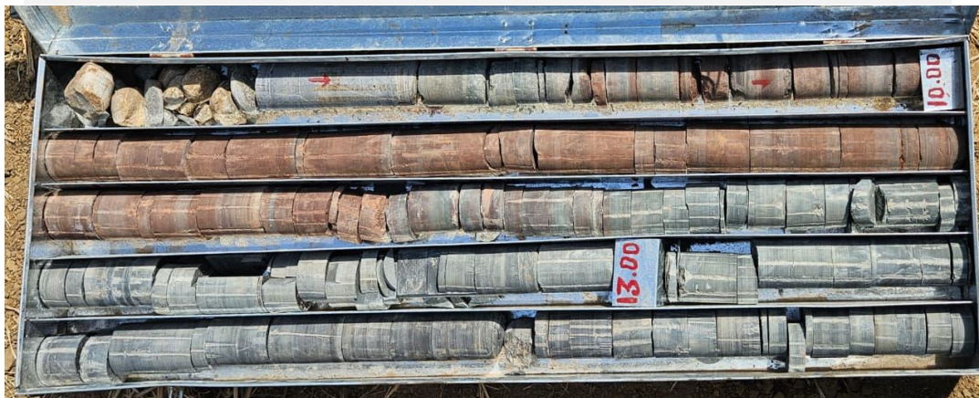
Photo.7.6: Core photograph showing Pindra shale, Boreholeno.MDLH-02
